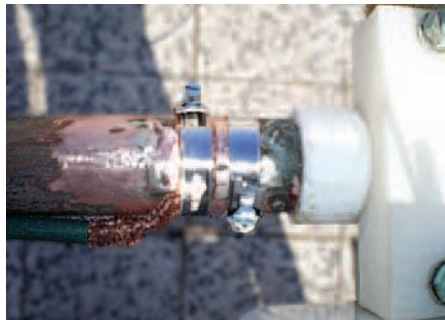
PHOTO 8: Using hose clamps to secure cables to the loop ends.
