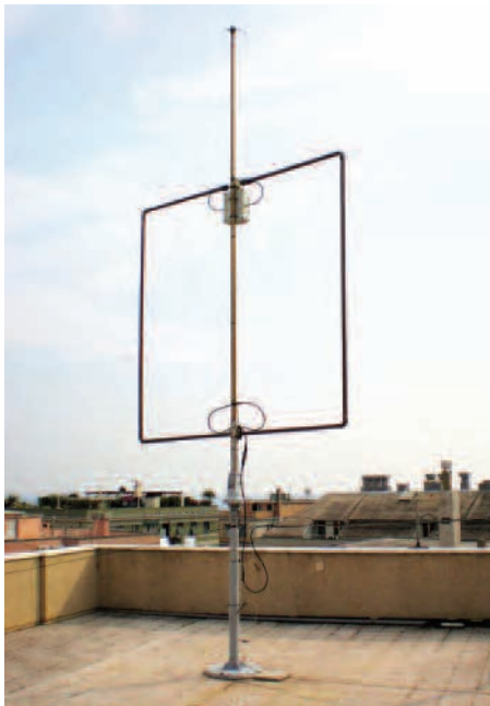
PHOTO 1: The refurbished loop for 160, 80 and 40m. The tuning unit is in the box at the top.
