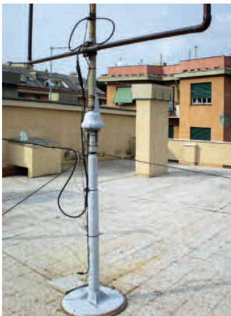
PHOTO 2: Prototype loop pedestal mount, rotator and feed.
