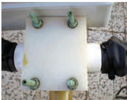
PHOTO 3: Detail of the Teflon bar connecting the loop frame ends.
