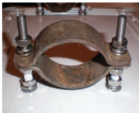
PHOTO 6: Detail of the collar flange on the back of the tuning unit box.
